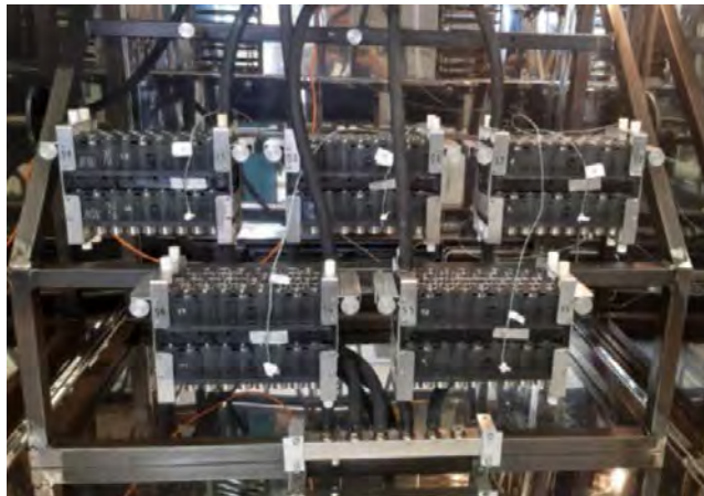
5 x 2S stacks (10 hollowblocks) with dummy cells (limiting samples), filled with cooling liquid at maximum steady system pressure ( P_{rel} = 1 \text{ bar} )
